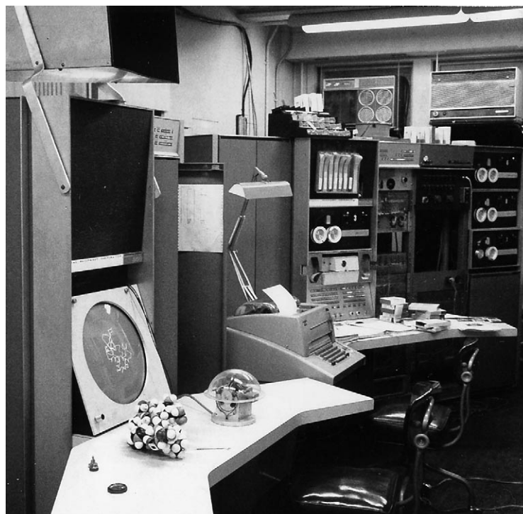
Figure 4. The second generation of hardware for Levinthal's molecular model building system: in the back, the PDP-7 mini-computer; in the middle, the standard teletype programming console; in the foreground, the DEC 340 graphics display console, with the 'globe' that served to control the direction and rate of rotation of the image. The space-filling model of an unspecified molecule stands next to the globe (courtesy of Martin Zwick).
